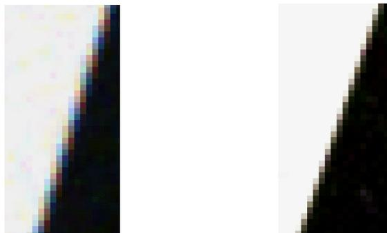
Figure 10: Real-world images obtained from cameras using the Bayer CFA on a CCD image sensor, (left) and the Foveon X3 image sensor (right).
