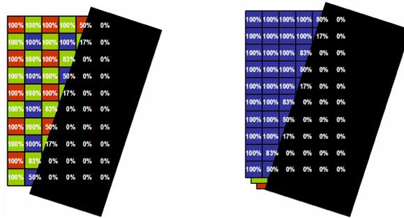
Figure 7: Bayer CFA image sensor, left, and Foveon X3 image sensor, right, with simulated edge superimposed. Percentages refer to percent response, based on percent of area exposed, equivalent to a 100% fill-factor pixel. Response normalized so that black = 0% and white = 100%. These percentages were scaled to 8 bits for simulated image output.
