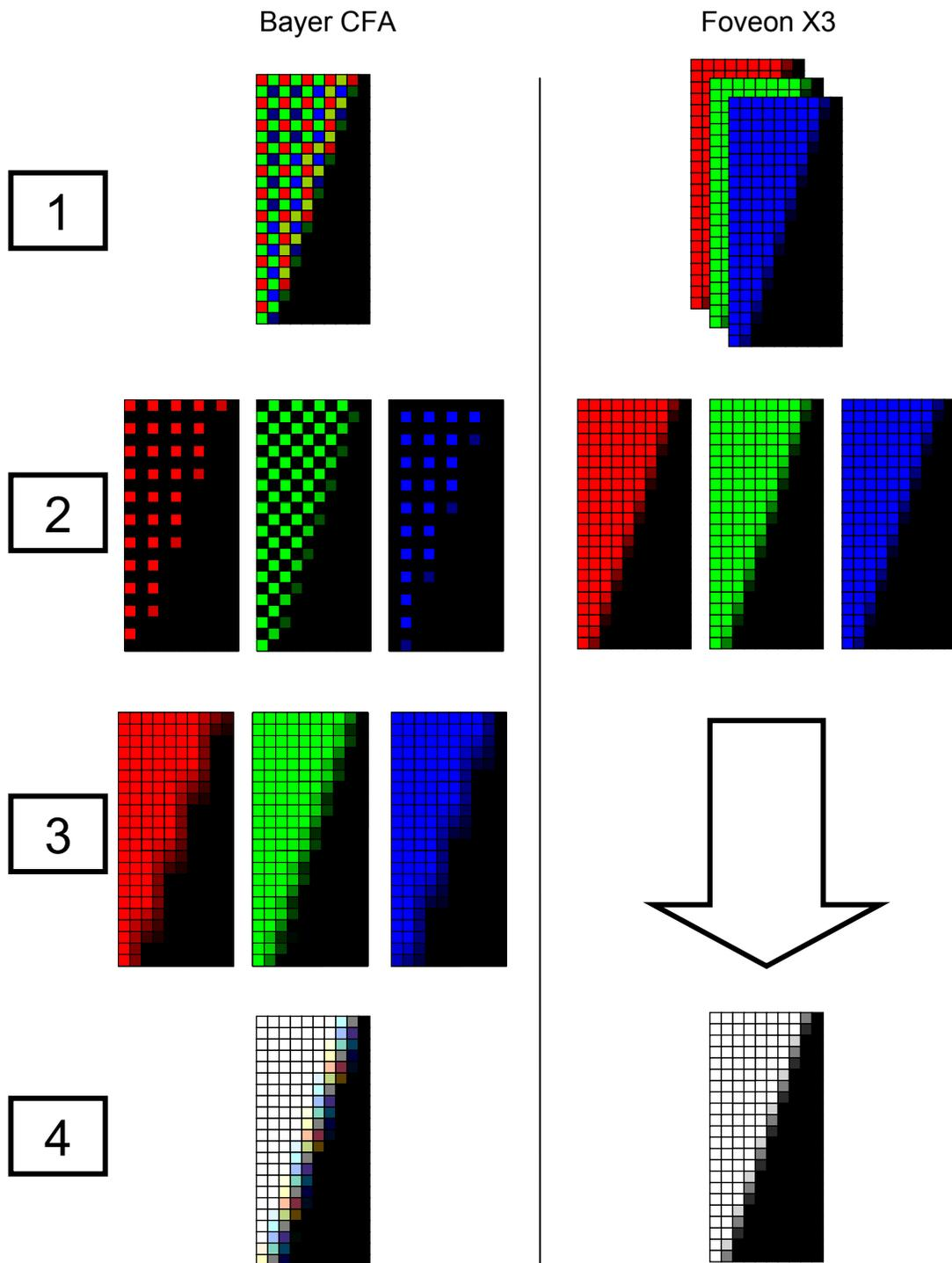
Figure 6: Comparison of color image capture planes and resulting images for a simulated edge.
