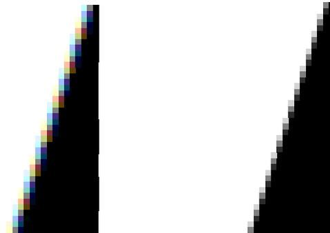
Figure 9: Simulated Bayer CFA (left) and Foveon X3 image sensor (right) responses to slanted edge. Note lack of colored artifacts and sharper edge in the X3 sensor example.
