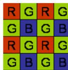
Figure 1: Typical Bayer CFA showing the alternate sampling of red, green, and blue pixels.
