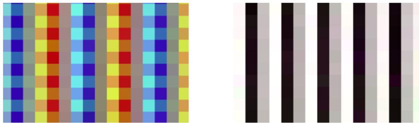
Figure 13: Digital camera output of a high frequency bar target (1/3 cycle/pixel location) for a Bayer image sensor (left) and a Foveon X3 image sensor (right).
