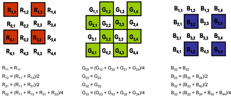
Figure 5: Bayer CFA color sample positions and the color interpolation equations used in this investigation
