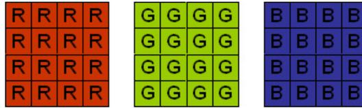
Figure 4: Fully populated image sampling found in film scanners, color-separation prism cameras, and also in Foveon X3 image sensors.
