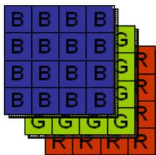
Figure 3: Schematic depiction of a Foveon X3 image sensor showing stacks of pixels, which record color channels depth-wise in silicon.
