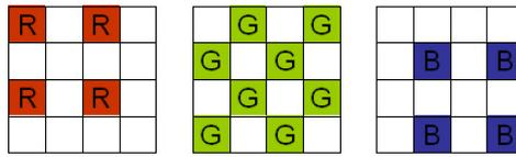
Figure 2: Decomposition of a typical Bayer CFA pattern into its components. Under-sampling in the image plane results in lower sharpness than could otherwise be achieved. Further, gaps in the image plane lead to color moiré artifacts.
