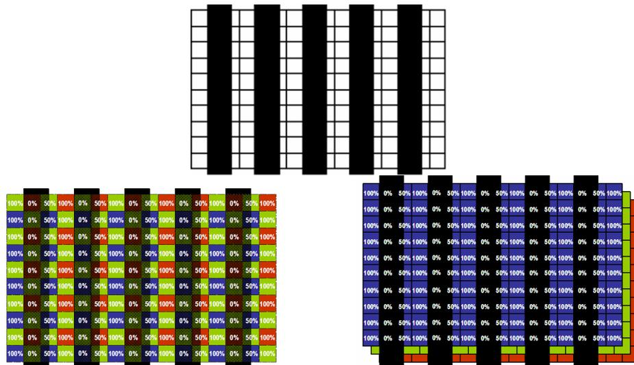
Figure 8: Bar pattern with frequency of 1/3 cycle/pixel location (top). Same bar pattern superimposed on Bayer CFA, left, and Foveon X3 sensors, right, with resulting relative responses (in percent).
