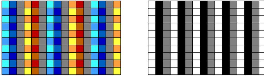
Figure 11: Simulated result of imaging a high frequency bar pattern on a Bayer CFA (left) and a Foveon X3 sensor (right).
